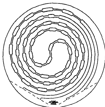
Figure 3 - Layout of flat-weighted chirp filter with 11.5 ns of dispersive delay and 14 ns of total delay. Klopfenstein-taper impedance transformers make the transition between the narrow 50-ohm input lines and the wider 40-ohm tapped delay lines.
